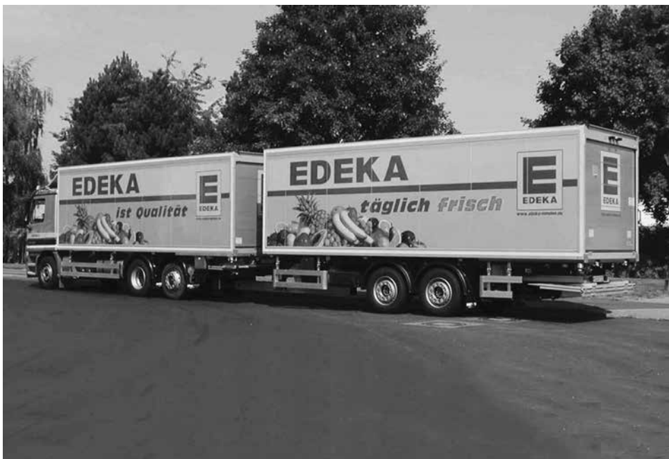
Figure 29.5 Close-coupled draw-bar combination
