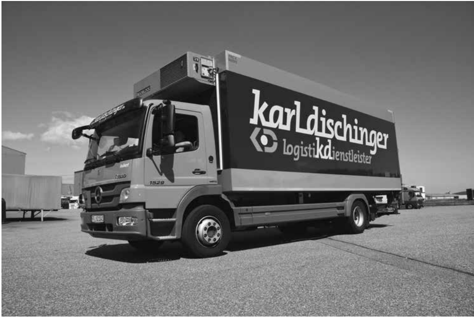
Figure 29.2 Four-wheeled rigid vehicle fitted with a refrigerated body
