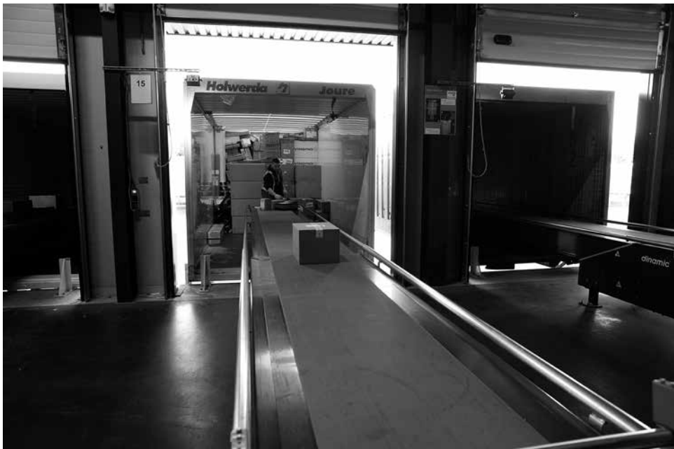
Figure 22.1 Telescopic boom conveyor
