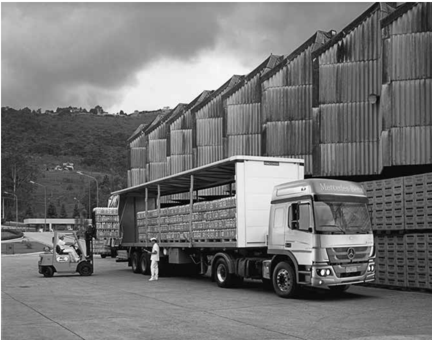
Figure 29.13 Curtain-sided trailer giving ease of access for loading
