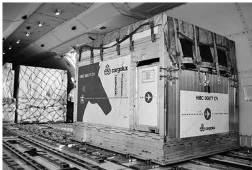
Figure 27.2 Cargolux air freighter being loaded using the powered rolling floor
