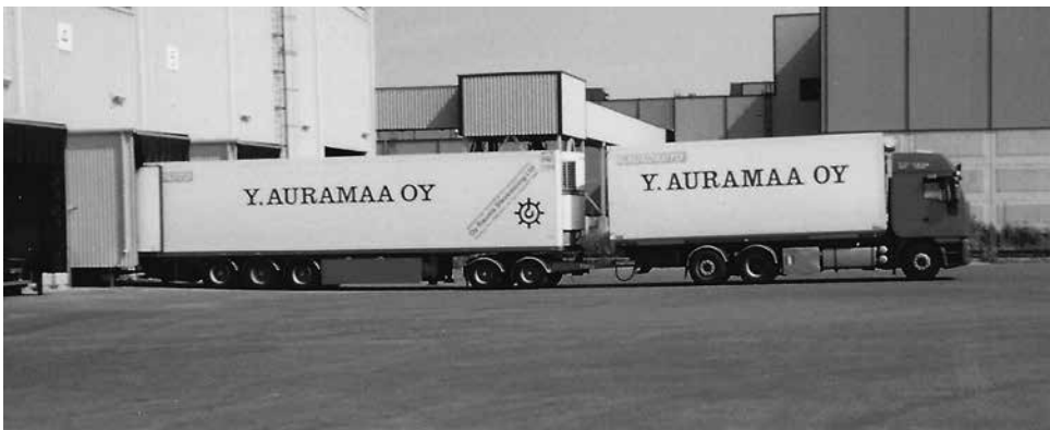
Figure 29.4 A 6×2 rigid vehicle towing a triaxle semi-trailer by means of a tandem axled bogie fitted with a fifth wheel coupling. Both vehicle and trailer are fitted with refrigerated bodies. Oulu, northern Finland
