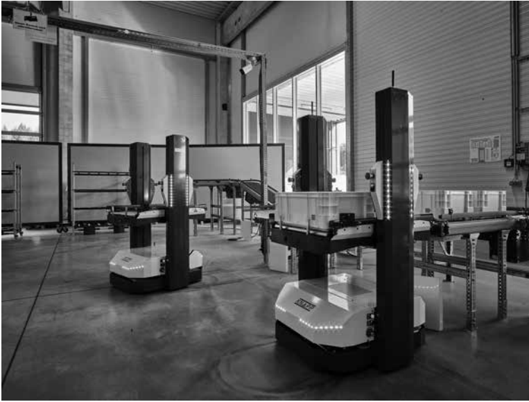
Figure 20.3 Autonomous mobile robots (AMRs) used for transporting tote bins
