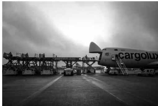
Figure 27.3 Air freighter being loaded through the nose with out-of-gauge cargo
