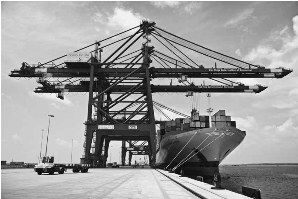
Figure 28.5 Ship-to-shore gantry crane loading a cellular container ship
