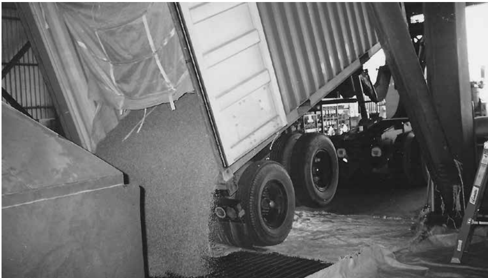
Figure 28.12 Container loaded with grain being unloaded by using a hydraulic ram to lift the trailer. The liner used to secure the grain inside the container can be clearly seen
