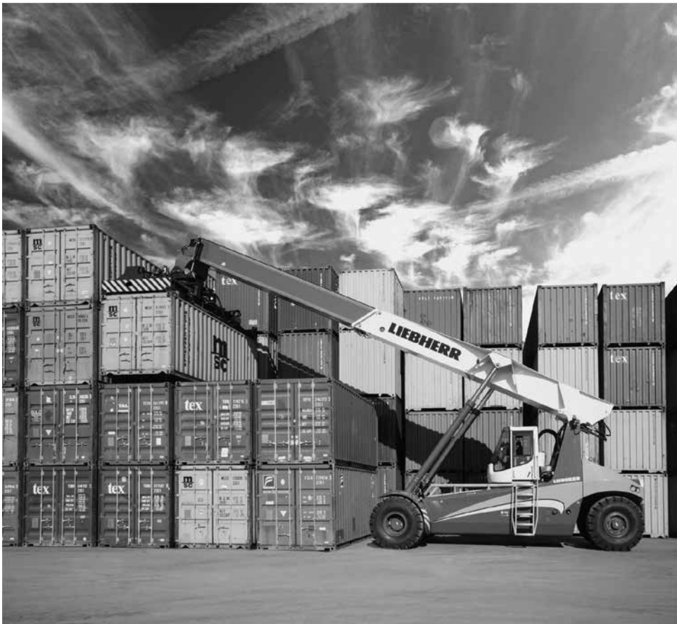
Figure 28.7 A reach stacker stacking ISO containers
