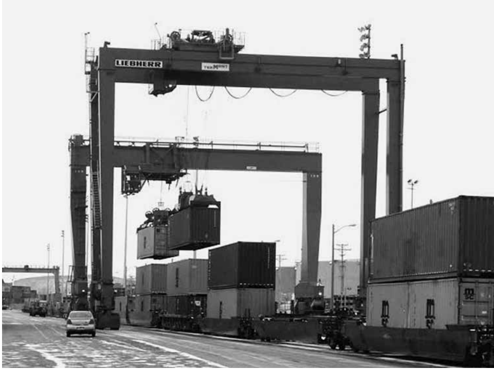
Figure 28.6 Two gantry cranes loading ISO containers on to railway freight wagons. Note the double-stacked containers as this is in Canada
