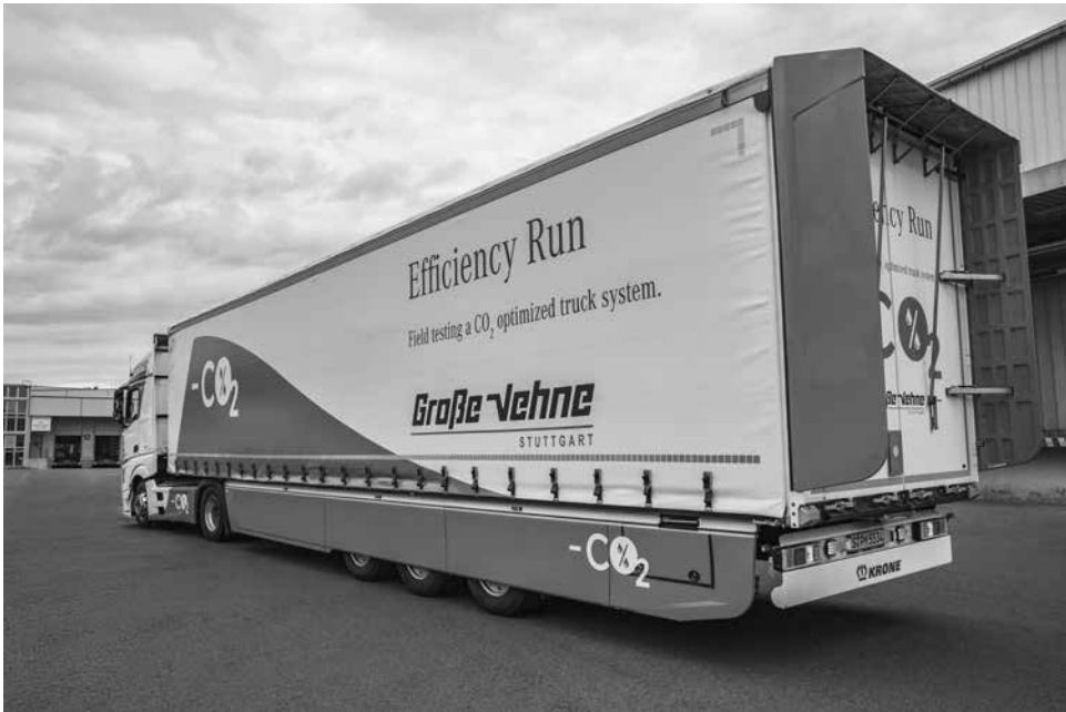
Figure 29.7 Articulated vehicle with a triaxle trailer equipped with aerodynamic mouldings to reduce drag and thus improve fuel economy
