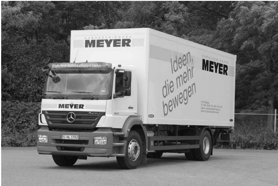
Figure 29.10 A 4×2 rigid vehicle equipped with a box body
