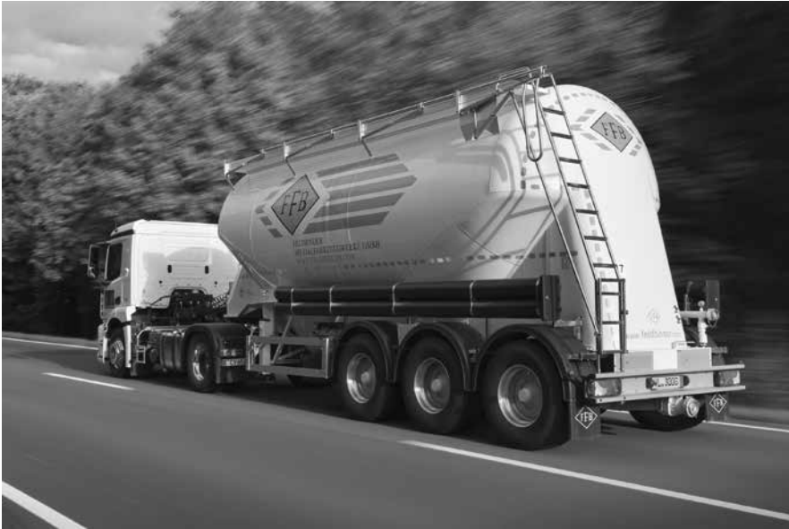
Figure 29.15 Triaxle Feldbinder bottom discharge tanker. The discharge pipe may be seen under the middle of the rear bumper bar
