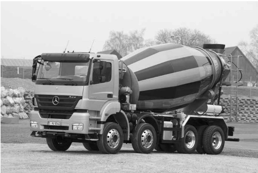
Figure 29.16 Eight-wheel rigid vehicle equipped with a cement hopper
