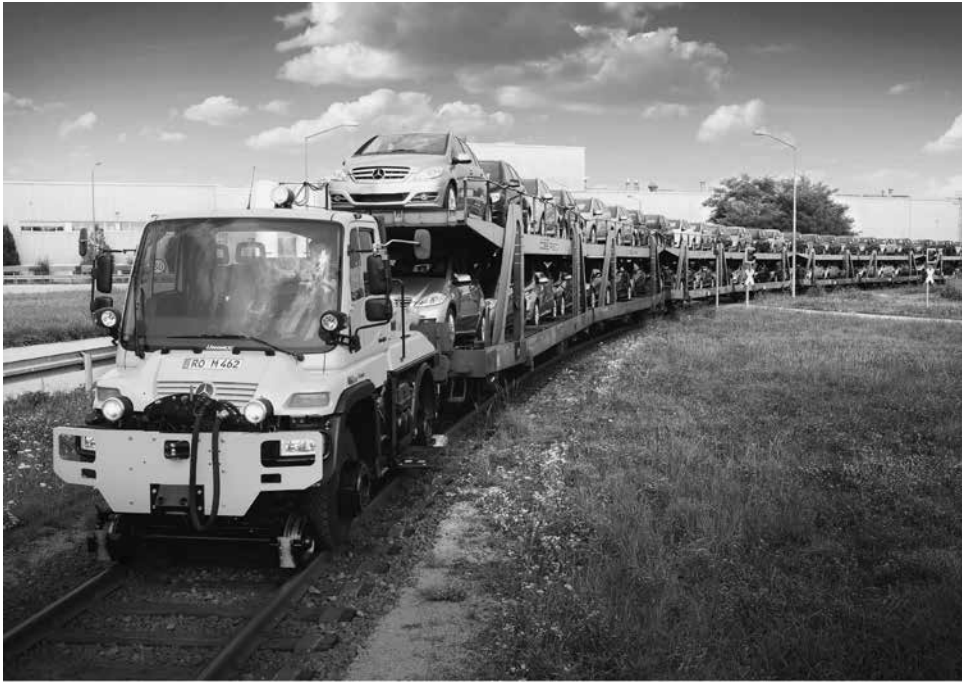
Figure 28.14 Double-decked rail cars loaded with new cars being towed by a converted road vehicle
