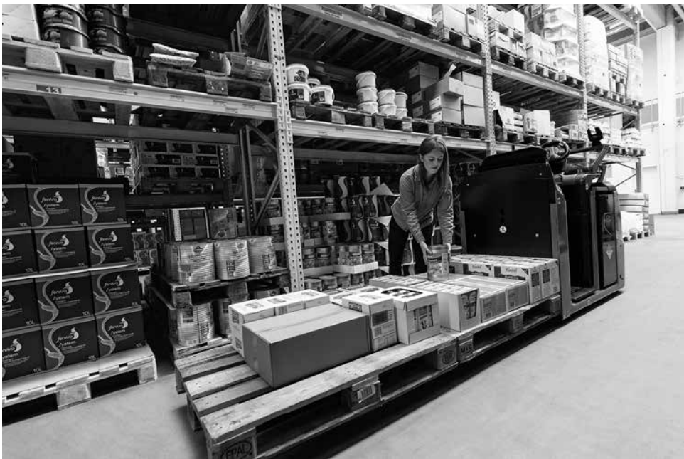
Figure 21.1 Order picking onto a low-level order picking truck (LLOP)
