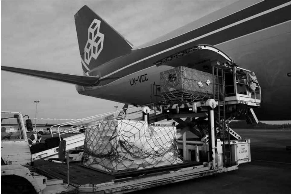
Figure 27.1 Air cargo pallets being loaded through the side door
