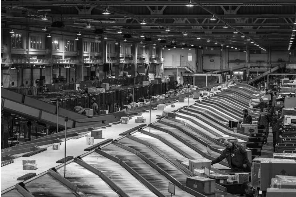
Figure 21.5 Sliding shoe sorter
