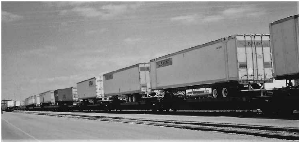
Figure 28.11 Road semi-trailers ‘piggybacked’ on rail cars in the United States
