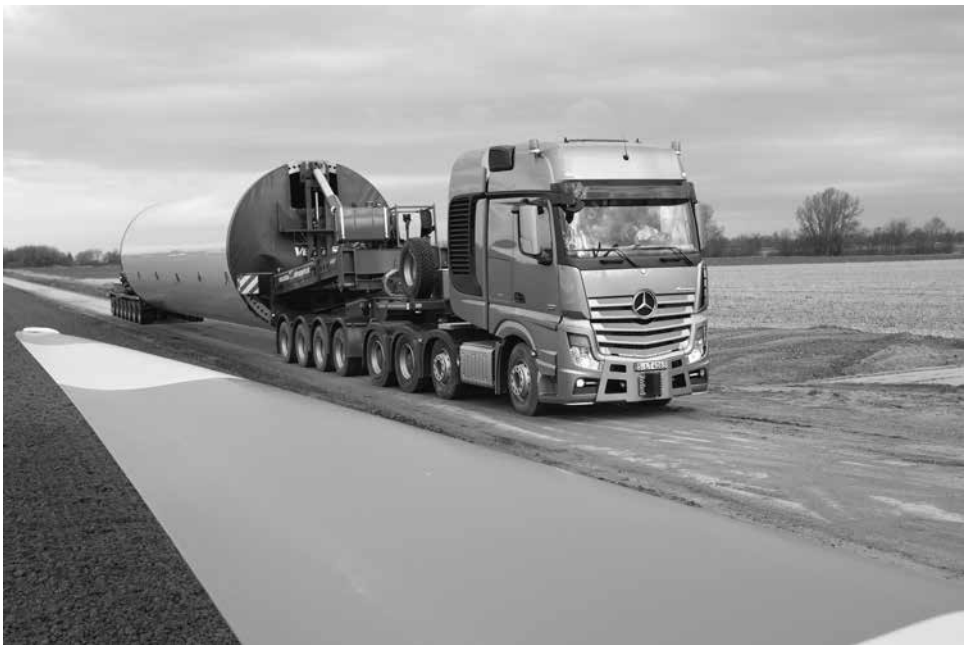
Figure 29.8 Heavy haulage tractor with an indivisible large load
