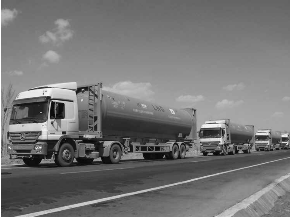
Figure 28.1 Articulated vehicle loaded with a tanktainer
