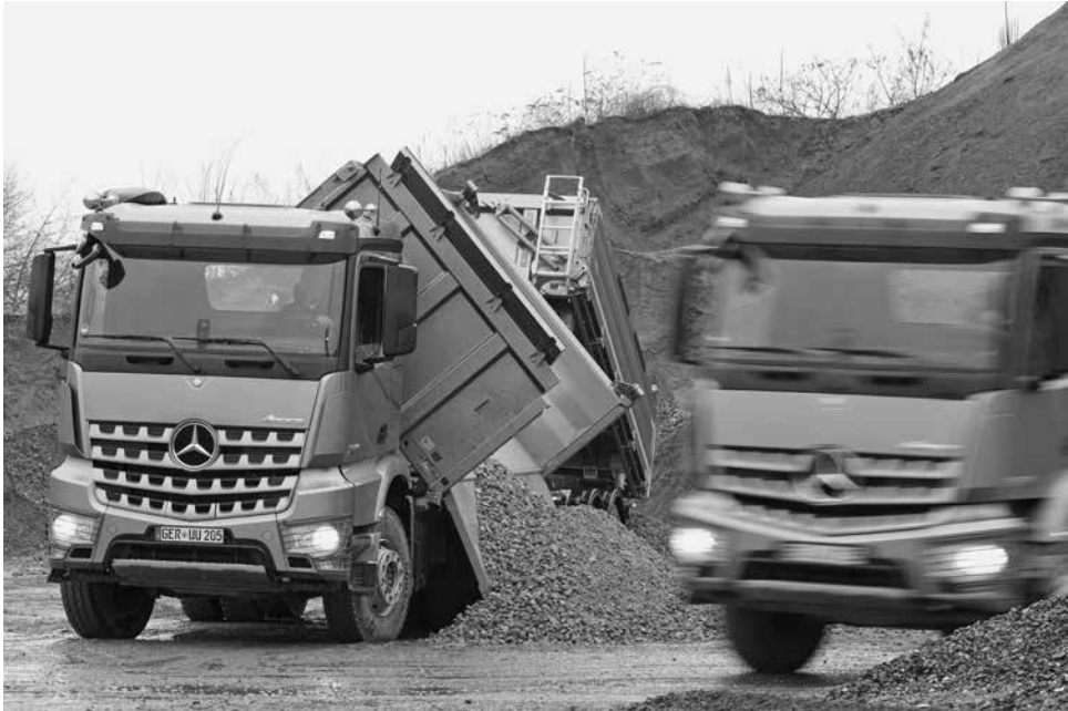
Figure 29.14 Vehicle showing tipping bodies. Note the fact that the vehicle is tipping one container to the side and the other container to the rear of the vehicle
