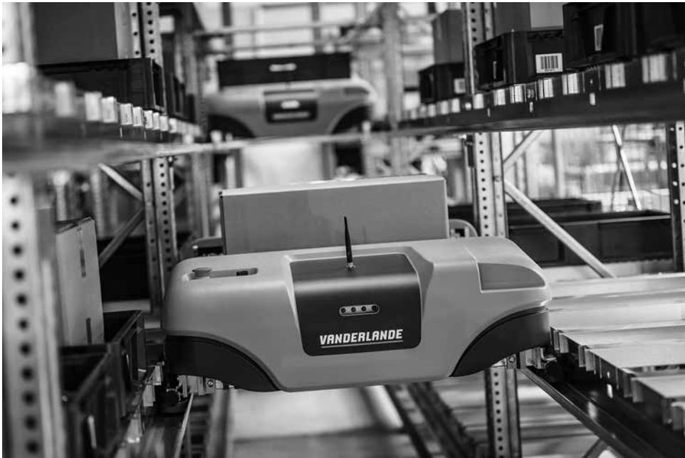
Figure 20.2 Miniload storage system with shuttles at each level
