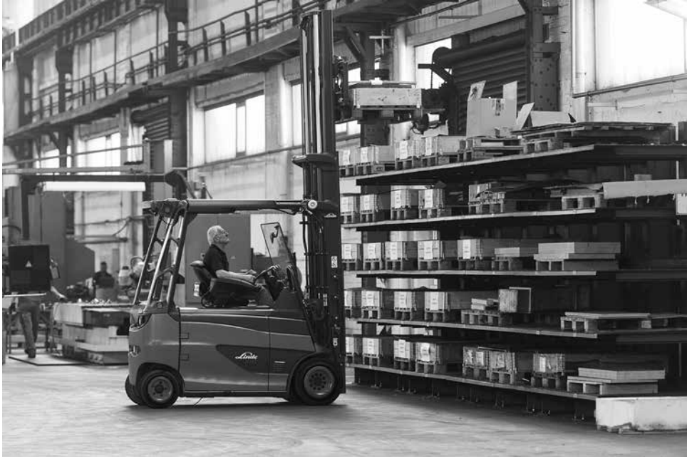
Figure 19.2 Electric counterbalanced fork-lift truck loading pallet into shelved cantilever racking
