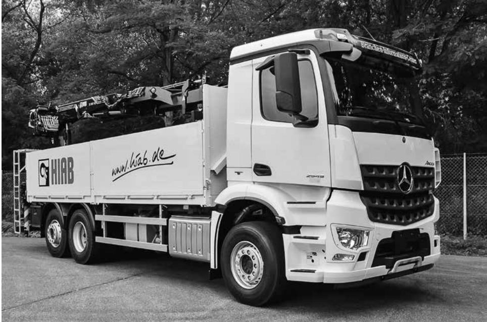
Figure 29.11 Platform or flat-bed 6×2 rigid vehicle with drop sides and HIAB crane to assist loading
