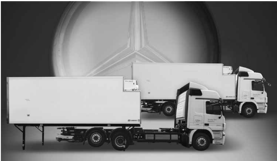
Figure 29.18 Demountable body system
