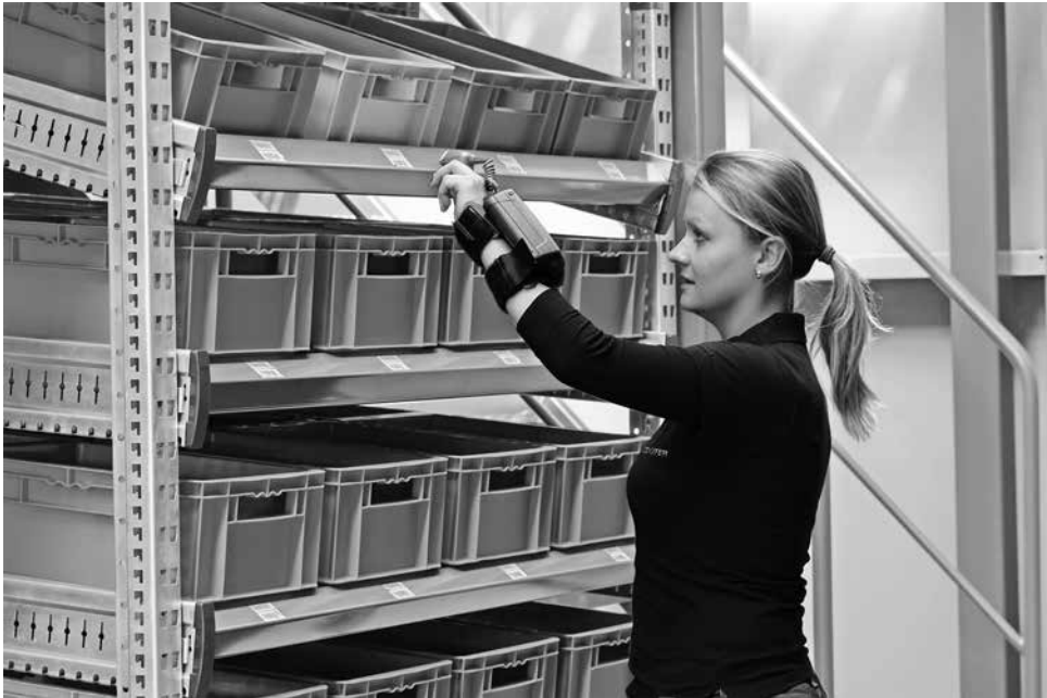
Figure 24.2 Barcode scanning using ring scanner and wrist-mounted radio data terminal
