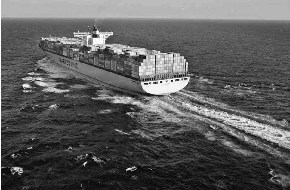
Figure 26.2 The Emma Maersk : one of the largest cellular container vessels in the world, capable of transporting 15,200 TEU
