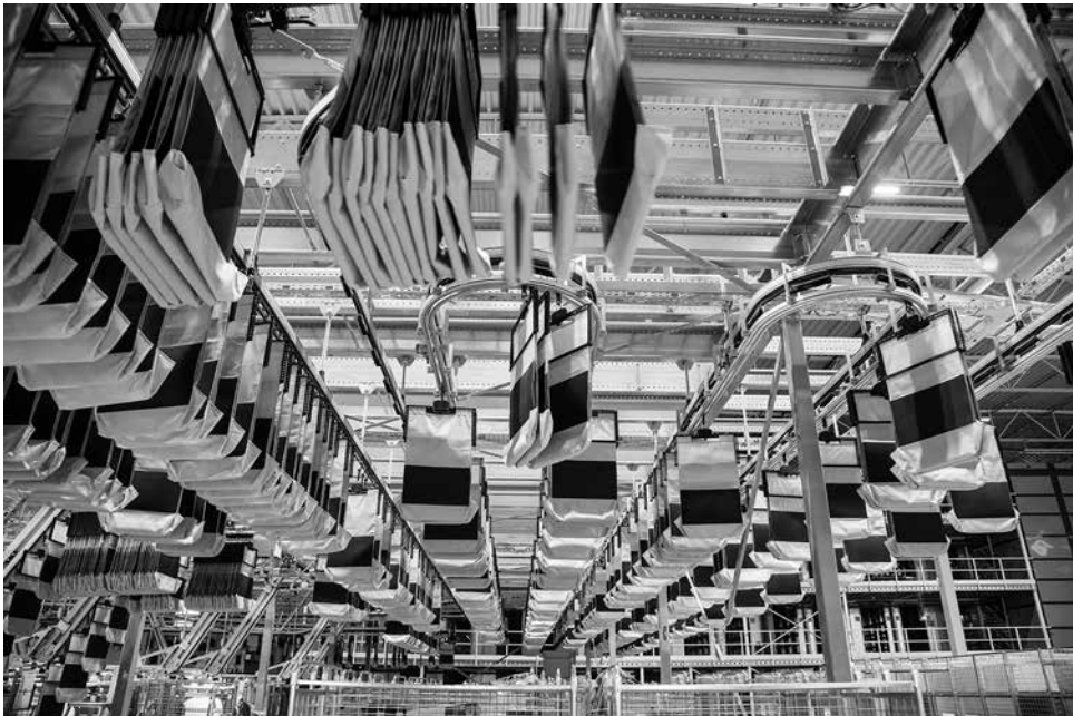
Figure 20.4 Hanging garment system that can also be used as a pocket sorter (described in Chapter 21)
