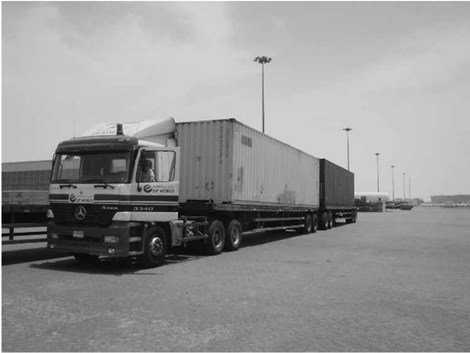
Figure 29.3 Double-bottomed articulated vehicle in Jebel Ali port, UAE
