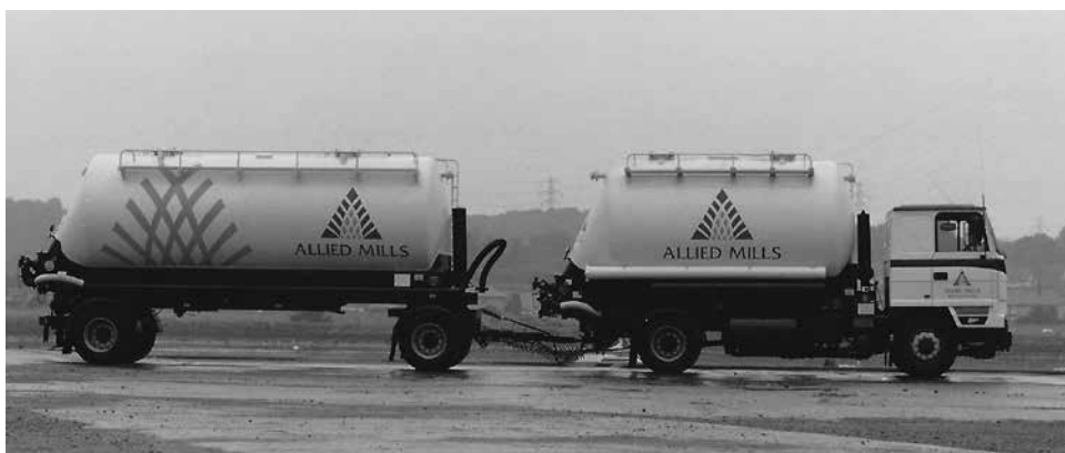
Figure 29.9 Rigid bulk powder tanker with a draw-bar powder tanker trailer
