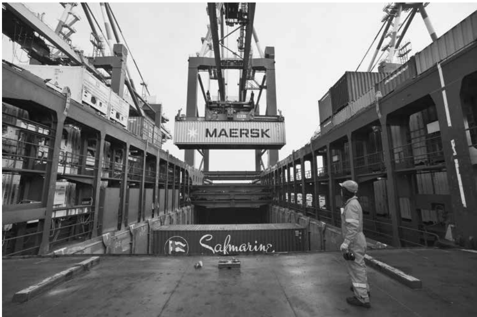
Figure 28.8 Containers being loaded into slots on a cellular container vessel
