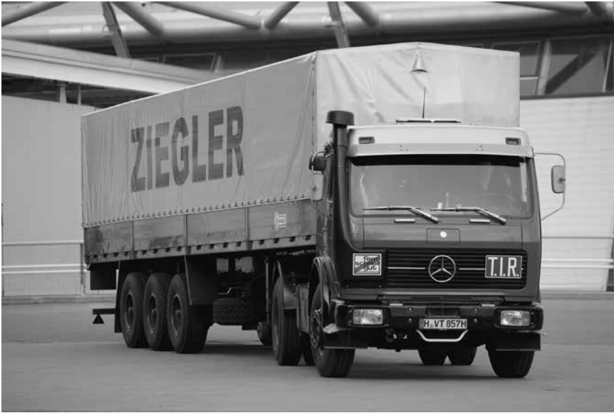
Figure 29.12 Articulated vehicle with a triaxle trailer fitted with a tilt body
