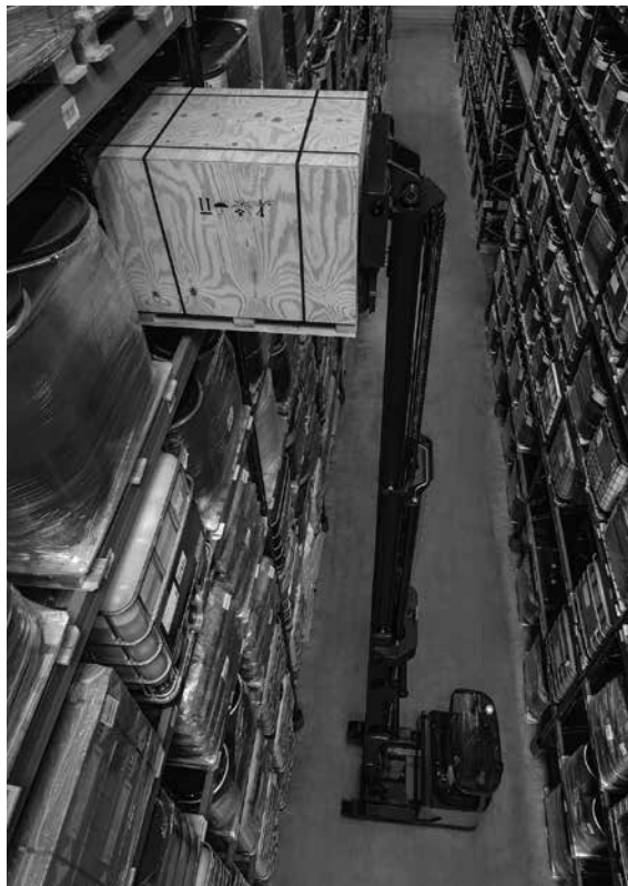
Figure 19.3 Reach truck working in aisle of adjustable pallet racking
