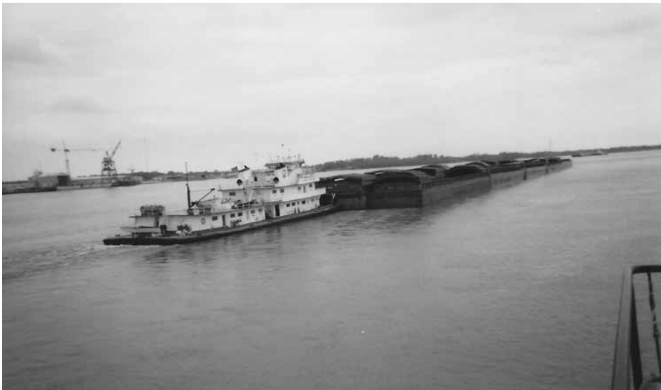
Figure 28.9 River barges being pushed by a powerful tug on the Mississippi River in the United States
