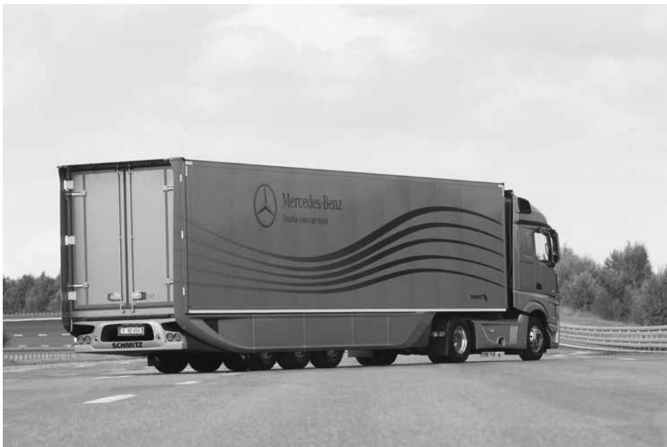
Figure 42.1 An articulated vehicle designed to be more aerodynamic
