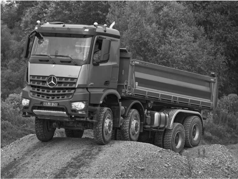
Figure 29.6 Eight-wheeled rigid tipper vehicle
