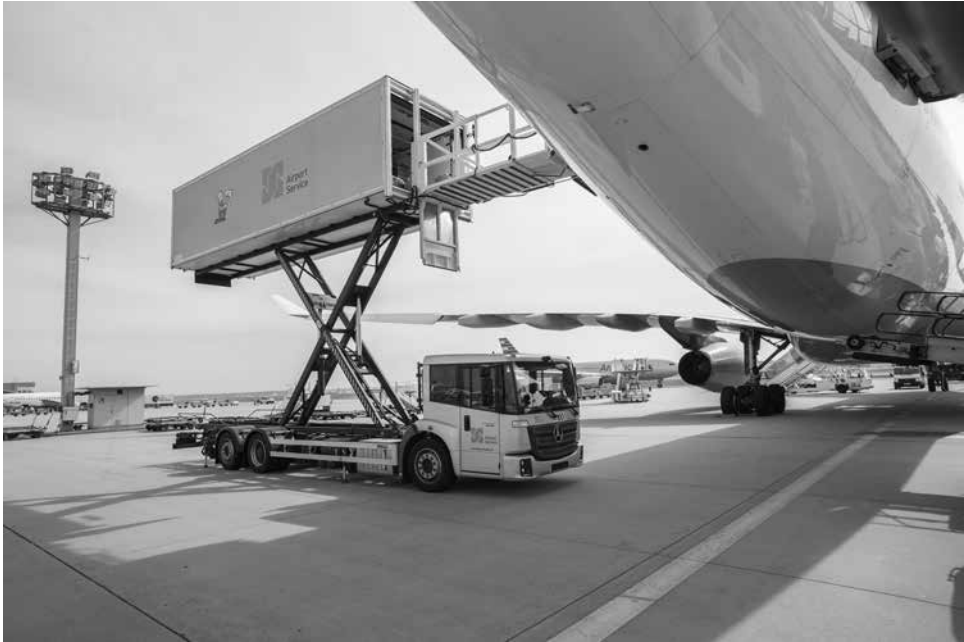
Figure 27.4 Aeroplane being loaded through the side door by a specialist vehicle equipped with a scissor lift
